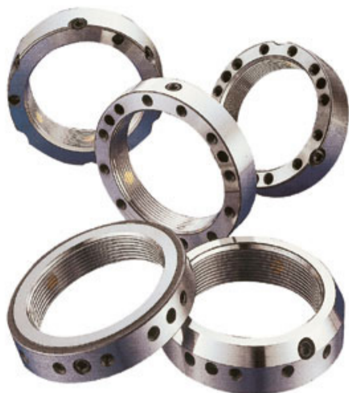
●材質：SCM440 ●硬度：HRC48°~52° ●ネジ精度：ISO4H
